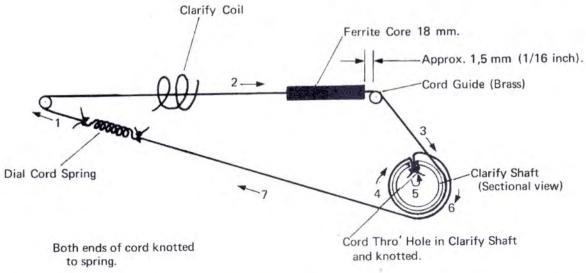
FRONT VIEW OF CLARIFY MECHANISM SHOWN WITH CLARIFY SHAFT FULLY CLOCKWISE.
